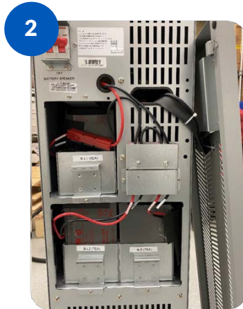
2 Lift up panel slightly and remove. Gently place off to side taking care not to dislodge ribbon cable.
